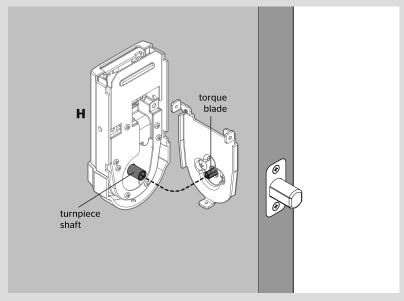
B Secure interior assembly with supplied screws.
