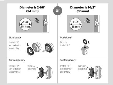
C Install exterior assembly and mounting plate.
