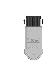
2 Press and HOLD the Program button while reinserting the battery pack.
