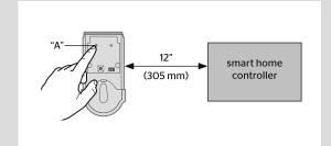
The lock and controller must remain stationary for at least 60 seconds during the pairing process.
