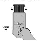
3 Press the Program button once more. When the LED flashes green and you hear two beeps, the lock has been reset.
